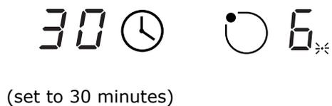
Touch the heating zone selection control, the corresponding timer will be shown in the timer indicator.
